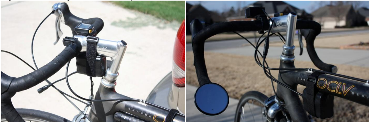
Typical Stand-Alone Headlight Battery Mounting Locations
